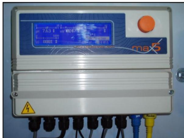
Figure 2. Multi-parametric Sensor for industrial wastewater prototype.
