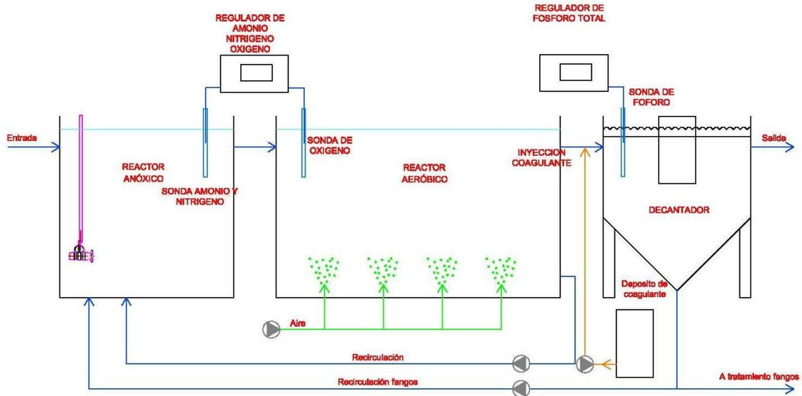
Figure 2. Scheme for urban wastewater prototype.
