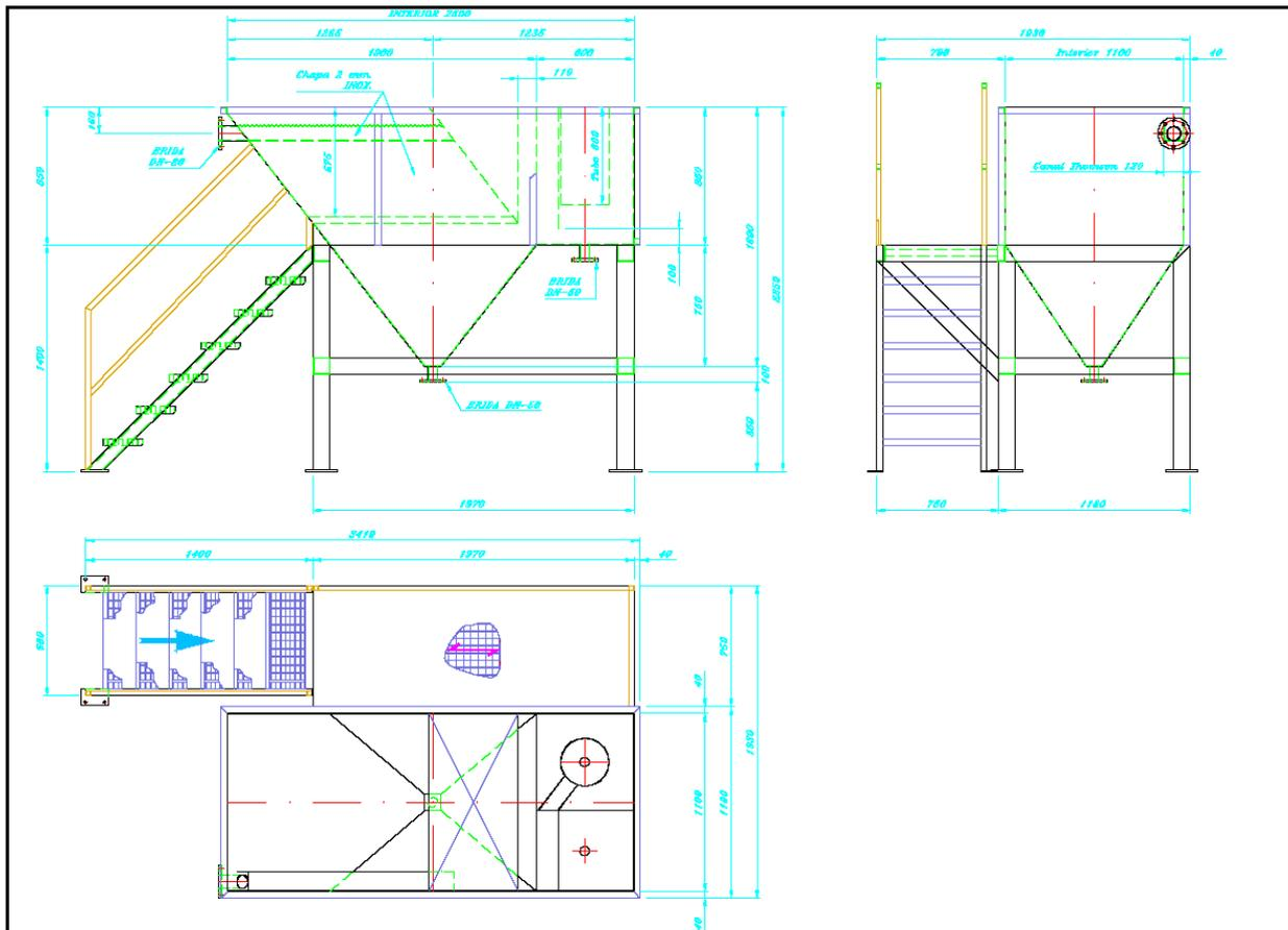
Figure 1. Scheme for industrial wastewater prototype.
